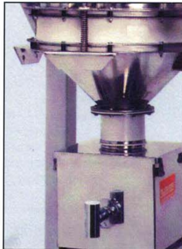
BAV 04 Series with FlexWall™ Feeder at Discharge.
