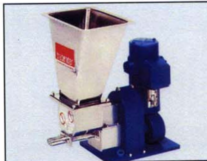
Feed Unit: Brabender MiniTwin Feeder
