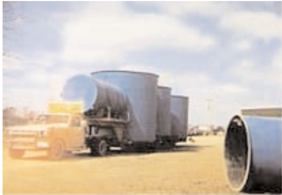
Various size open top, flat bottom tanks for beef processing plant
