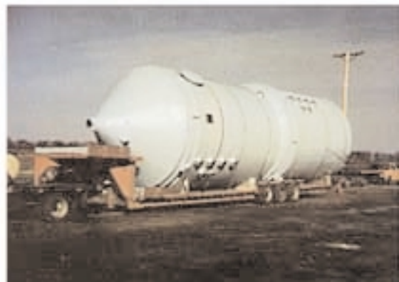
12' Cone Bottom tanks with legs removed from ring for shipment.
